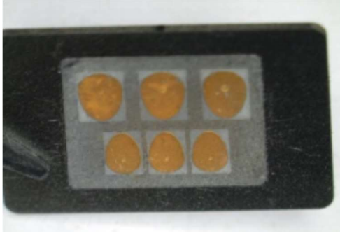
Figure 6: TTV chip manually assembled inside a titanium pocket before laser welding
