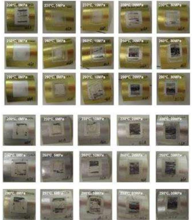
Fig. 4 - Mandrel bend test results.
